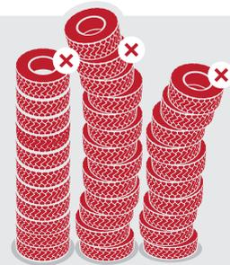
**DON'T** stack stock or store in a way that any forces may cause compression or permanent distortion
