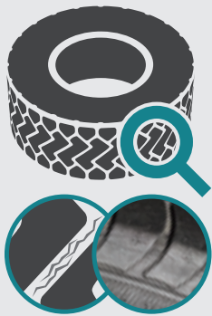
Cracking between tyre tread
