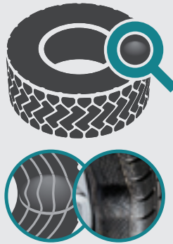
Bulten in de bandwand
